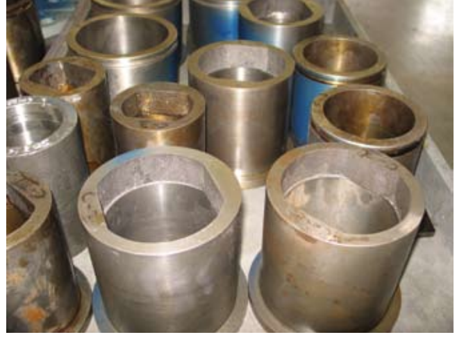
Pump shaft sleeves ready to be loaded into a cryogenic processor.
