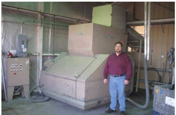
Dave Waller, maintenance superintendent at Rantoul Products, stands beside a large granulator equipped with cryogenically-treated blades.
