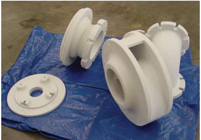
Pump components (frosty from cold) removed from a cryogenic processor for a few minutes for inspection.
