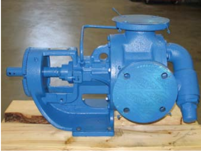
A pump housing on a pallet prepared for loading into a cryogenic processor.
